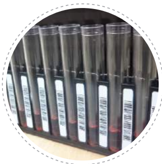
Sample strip loading rack with bar code reader (left side)
